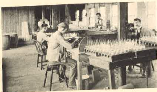
Putting exhaust stems on refilled bulbs.
